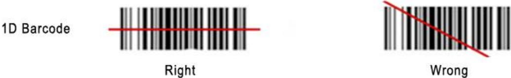
**Figure4.1-3 1D Barcode Scanning**
